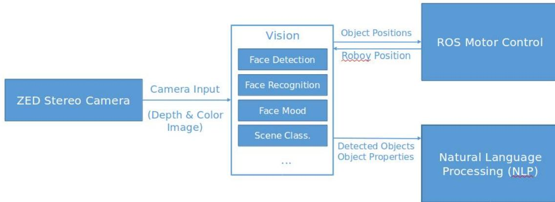
Fig. 1.1: **Context diagram** - shows the birds eye view of the vision system (black box) described by this architecture within the ecosystem it is to be placed in. Shows orbit level interfaces on the user interaction and component scope.
